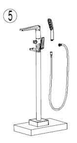
5. Flush any contaminates in supply lines for 30-60 seconds until water is clean. Then, fix the assembled faucet to the seat (8).
