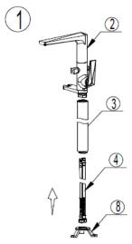
1. Put the inlet flexible hose (4) through faucet tube (3), and fix the inlet hose (4) to bath faucet (2). Then fasten the fixing seat (8) to the faucet tube (3)
