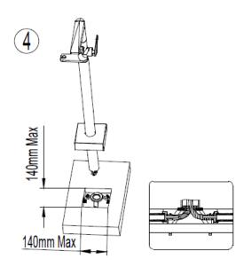
4. Drill out the hole as per the marked position, then fix the explosion screws (7) and fasten to the fixing seat (8).
