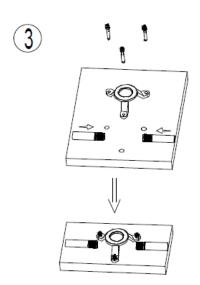
3. Drill out the hole as per the marked position, then fix the explosion screws (7) and fasten to the fixing seat (8).
