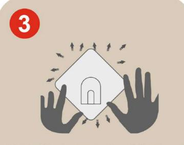
Stick the SRS adhesive pad on the wall. Rub the pad and press firmly. If there are any air bubbles, remove them by rubbing over towards the edge.
