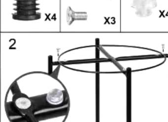
Please distinguish the front and back of the ring before installing the screws.
