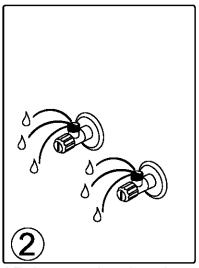
2.Flush any contaminates in supply lines for 30-60 seconds until water is clean.
