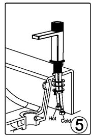
5.screw out the thread pipe from the fasten parts (3), and then tighten the thread pipes to the faucet.
