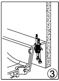
3.Pass all the fasten parts (3) in correct directions through the hot & cold inlet hose (5), then make these hose (3) go through the hole from down to top counter.
