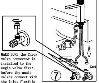
7.Install the Check valve connector(9) to angle valves linked with Hot & Cold water supply pipe, then fasten it by spanner to the other end of the Hot & Cold Inlet flexible hose(5).
