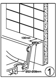
1.Make a hole on the counter at Φ32 - Φ38mm
