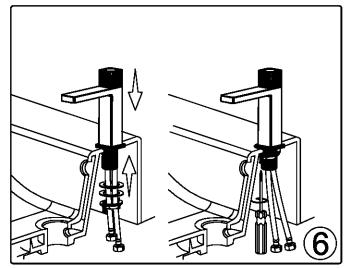
6.Fasten the screws nut from (3) with screwdriver.
